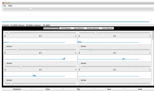
Figure 2: A snapshot from the interface provided with the tool. The upper part presents the initial level design which is modified in realtime to provide visual feedback about designer’s choices. Patterns of different components are presented in the lower frames. The designer can activate/deactivate each pattern and change its weight and edits will be directly reflected in the upper frame.
